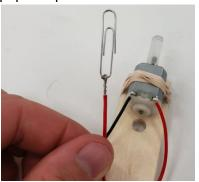
**Step 6.** Connect the red wire of the battery pack (#4) and the black wire of the motor (#3) together by twisting the metal together.
