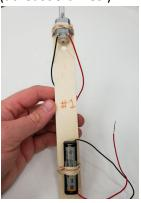
**Step 4.** Wrap the exposed metal wire from the black wire of the **BATTERY PACK** (#4) around the bottom of one paper clip (#6) so that the wire holds onto the paper clip.
