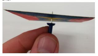
**Step 10.** Push the pushpin into the glue stick attached to the motor (#3).
