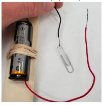
**Step 5.** Wrap the exposed metal wire from the red wire of the **MOTOR** (#3) around the bottom of one paper clip (#6) so that the wire holds the paper clip to it.
